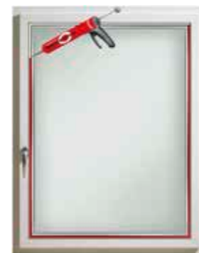
The remaining gap between glass and frame is filled with glue all around.
