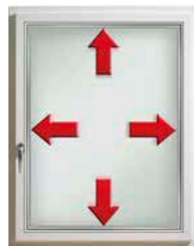
The glass pane is set into the frame and centred.
