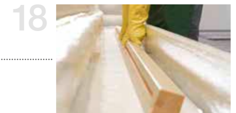
18 Impregnation of the timber parts ensure long life, best quality and optimum protection for all edges.
