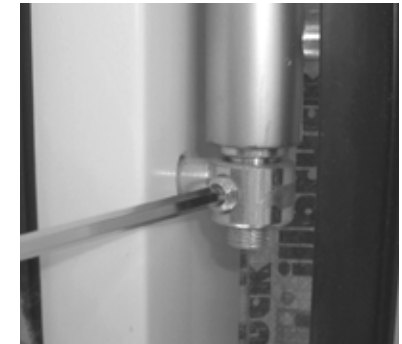
Loosen fixing screw.
